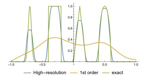
Figure 1: Comparison of exact solution (green) with numerical solutions obtained with fully implicit first-order accurate scheme [3] (orange) and the new TVD second-order accurate semi-implicit scheme (blue) for linear advection with constant speed after one period with Courant number equals 4 and h=2/500. Example taken from [5].
