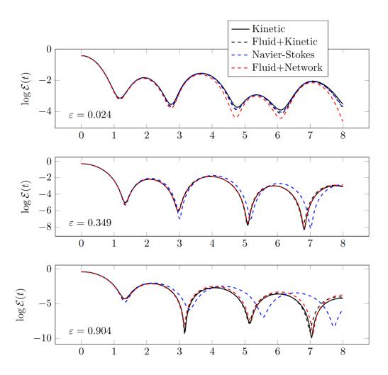
Figure 1: Electrical energy of the plasma in function of time, for different models: the kinetic model (Kinetic), and the fluid model using either the exact closure (Fluid+Kinetic), the Navier-Stokes closure (Navier-Stokes) or our network based closure (Fluid+Network).  $\varepsilon$  denotes the Knudsen number.
